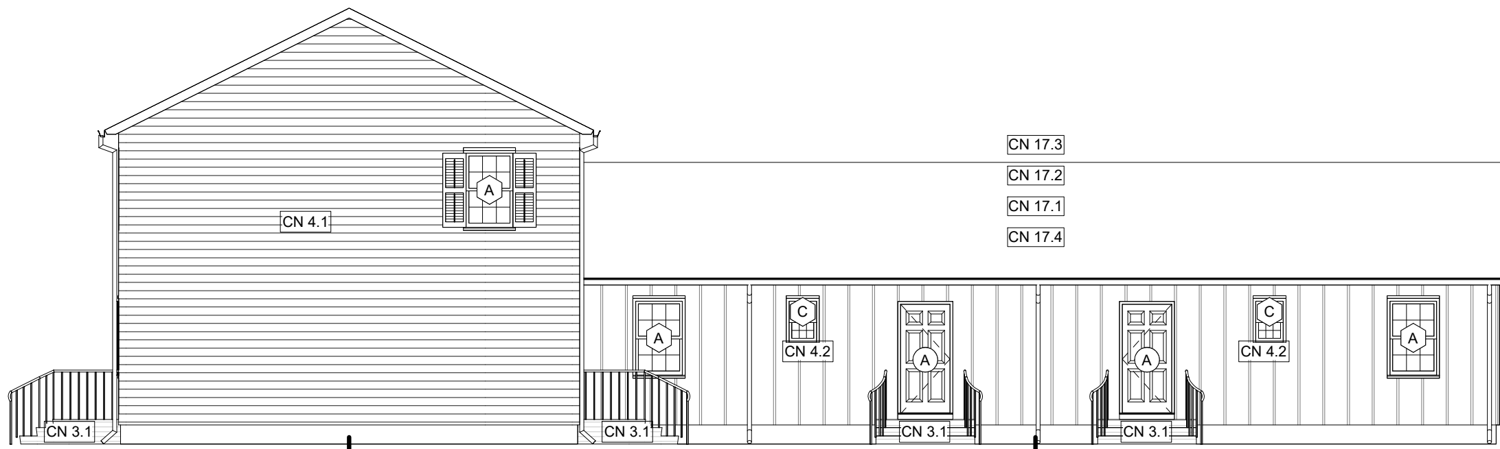
4 REAR ELEVATION - DEMO / NEW_BLDG TYPE XI 1/8" = 1'-0"
